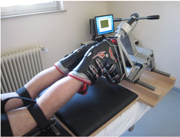
Fig. 2 Device used for the static rotational knee laxity measurements
