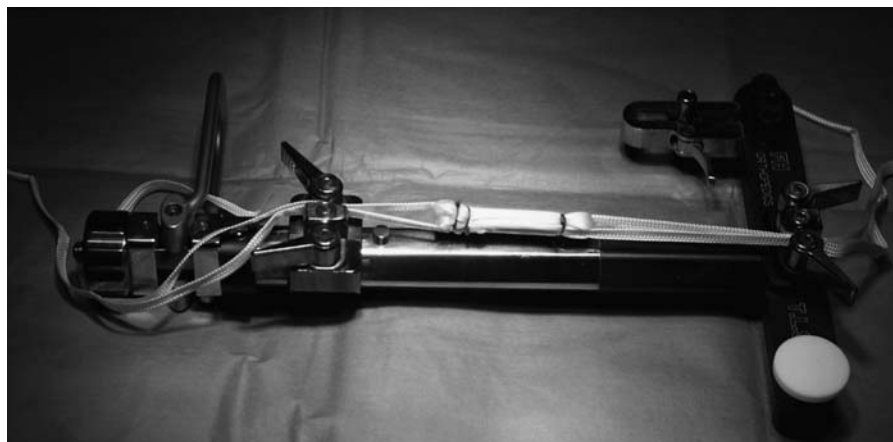
FIGURE 3. Semitendinosus folded into 4 strands on polyethylene terephthalate tapes put under tension on a table at 250 N.
